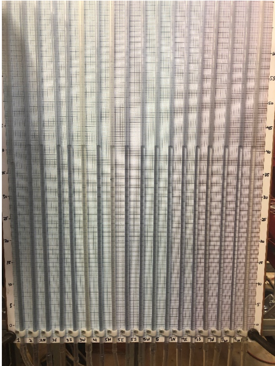
Figure 14. Manometer board attached to seepage flux tank.
