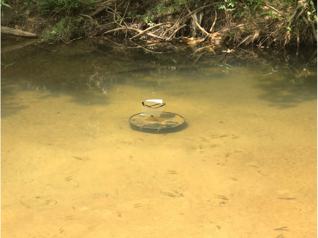
Figure 3. Half-barrel seepage meter installed in Goodwin Creek, Batesville, MS.
