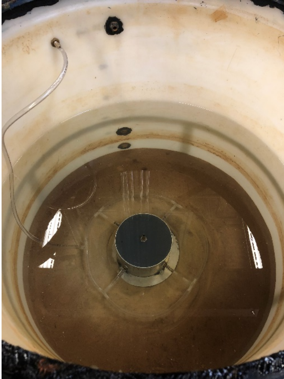
Figure 15. Scale model seepage meter placed in seepage flux tank.
