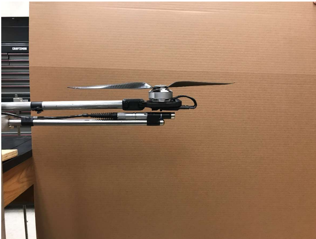
Figure 3.3. Experimental setup for non-rigidly attached microphone.
