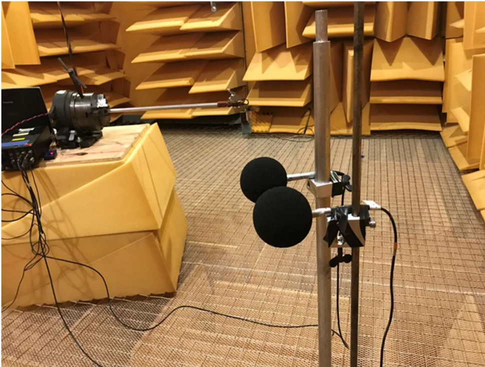
Figure 3.13. Double microphone setup in anechoic chamber.
