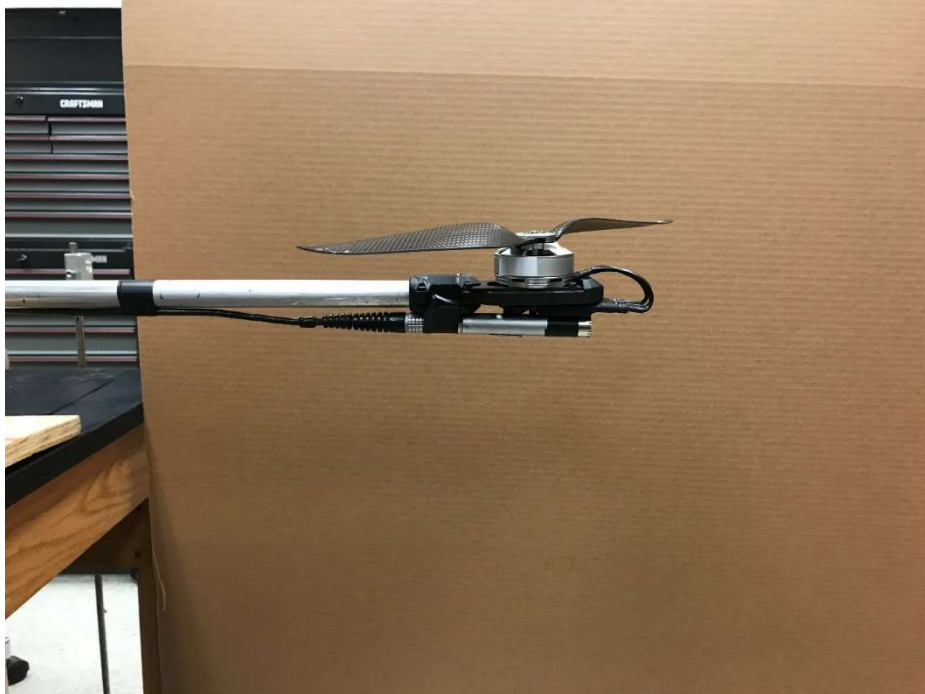
Figure 3.1. Microphone attached to the motor housing
