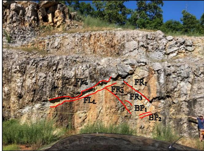
**Figure 5-2.** Road cut with measured surfaces for discontinuity survey labeled.
