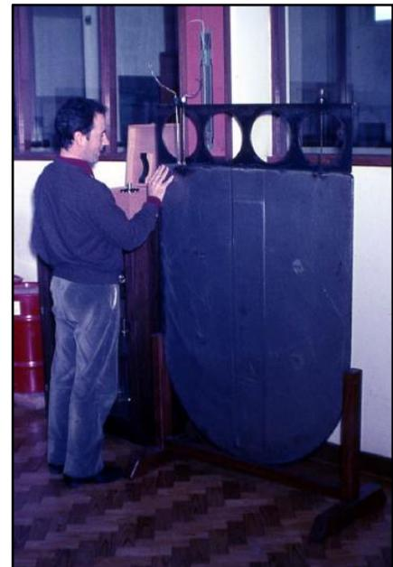
**Figure 2-18.** Flat jack to be inserted into rock mass (Hoek and Diederichs, 2006).
