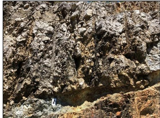
**Figure 5-5.** Kaolin infill of the fault.
