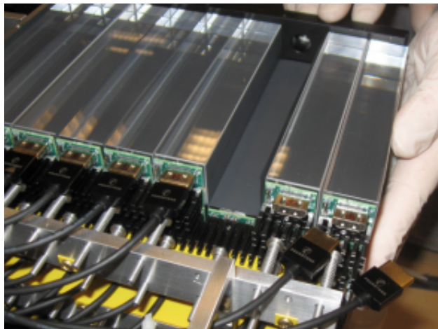
(b) A close view of the \text{PbF}_2 crystals connected to SiPMs at the end in order to collect the Cerenkov light from the positron hits
