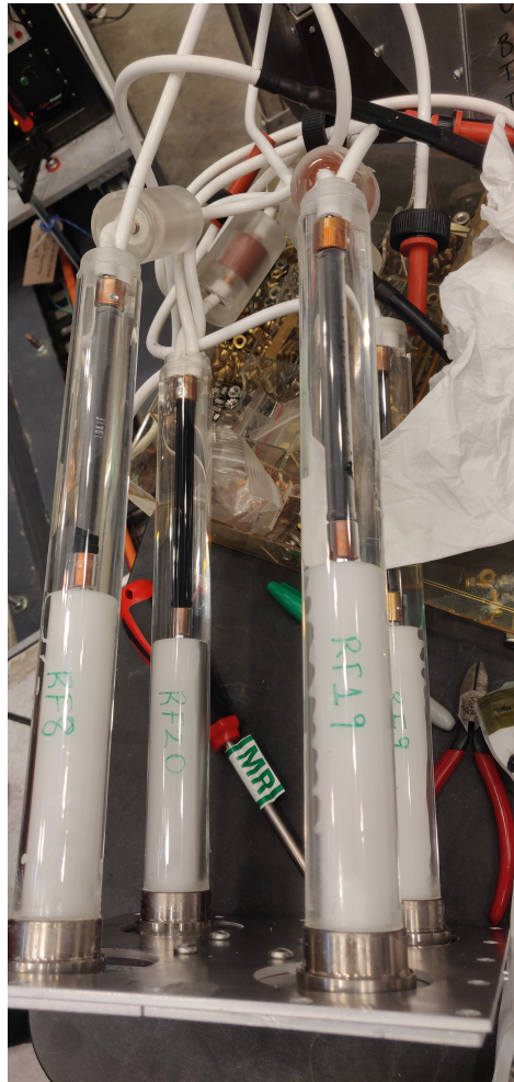
Figure A.7: Potted RF resistors that are now installed in all of the eight quadrupole systems
