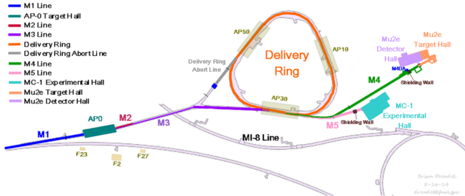
Figure 2.1: The schematic of accelerator beam-line components Fermilab uses to provide spin-polarized muon beam to E989. Protons start in the Linac, travel around the Booster and then the Recycler Ring, hit the nickel-based target at AP0, and produce pions. The pions then decay to muons in the Delivery Ring before reaching the muon campus [42].
