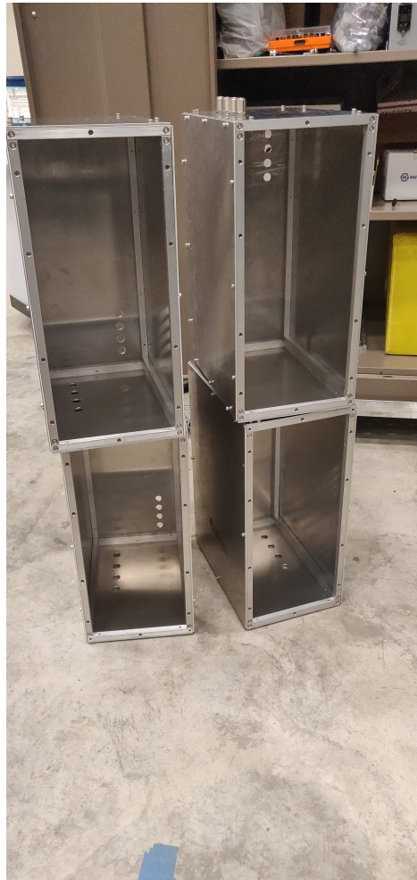
Figure A.6: RF extension boxes once assembled at MC-1
