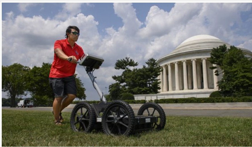
UM geological engineering graduate student Kristian Macias uses a ground-penetrating radar unit to collect data near the Jefferson Memorial in Washington, D.C. Photo by Thomas Graning/Ole Miss Digital Imaging Services
