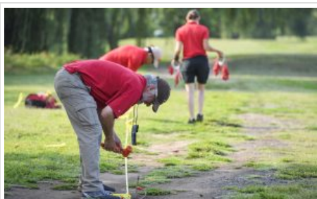
Greg Easson, director of the Mississippi Mineral Resources Institute and a UM professor of geology and geological engineering, helps the research team set up cables for an electrical resistivity tomography analysis at the East Potomac Golf Course. Photo by Thomas Graning/Ole Miss Digital Imaging Services
