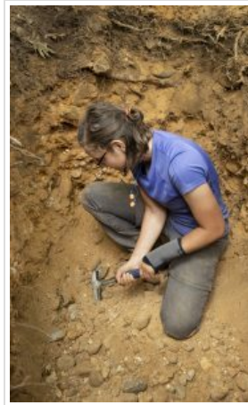
Graduate student Jodi Messick digs for gravel samples at the bottom of a hand-dug hole at the Smithsonian National Zoo in Washington, D.C. The sample is being sent to the U.S. Geological Survey laboratory in Denver for age dating. Photo by Logan Kirkland/Ole Miss Digital Imaging Services
