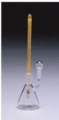
Figure 3.3. Image of pycnometer for measuring wax/n-heptane density.
