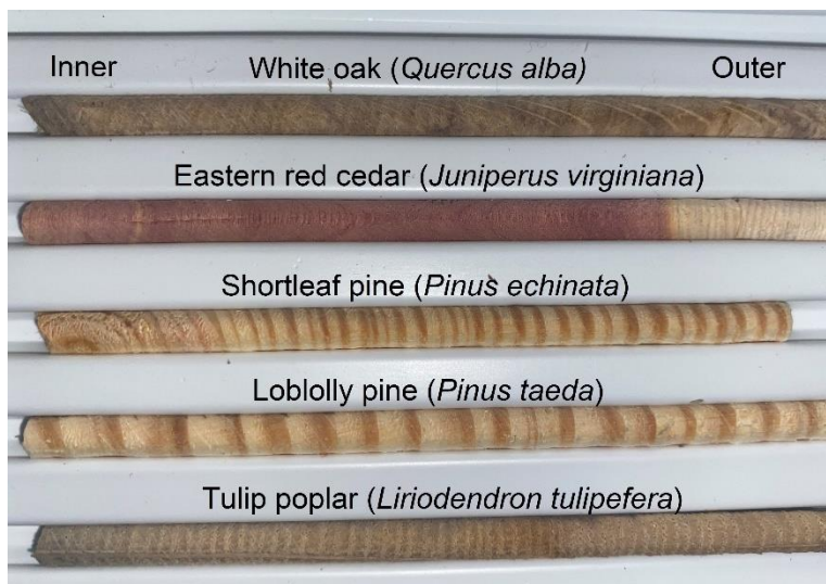
Figure 17. Example of tree cores collected with a 5.15-mm increment borer.
