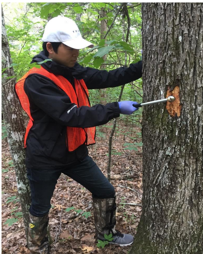
Figure 15. Tree core sampling using a hammer type borer
