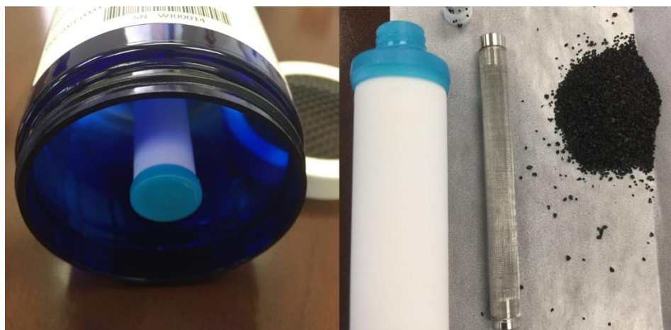
Figure 3. Photos showing the Hg passive air sampler (MerPAS) with a White Radiello diffusive body inside a protective shield and the mesh cover in the background (left), as well as a close up of the diffusive body, stainless-steel mesh screen, and sulfur-impregnated activated carbon sorbent (right).
