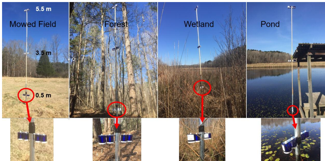
Figure 4. Deployment of Hg passive air sampler at the University of Mississippi Field Station during winter 2019.
