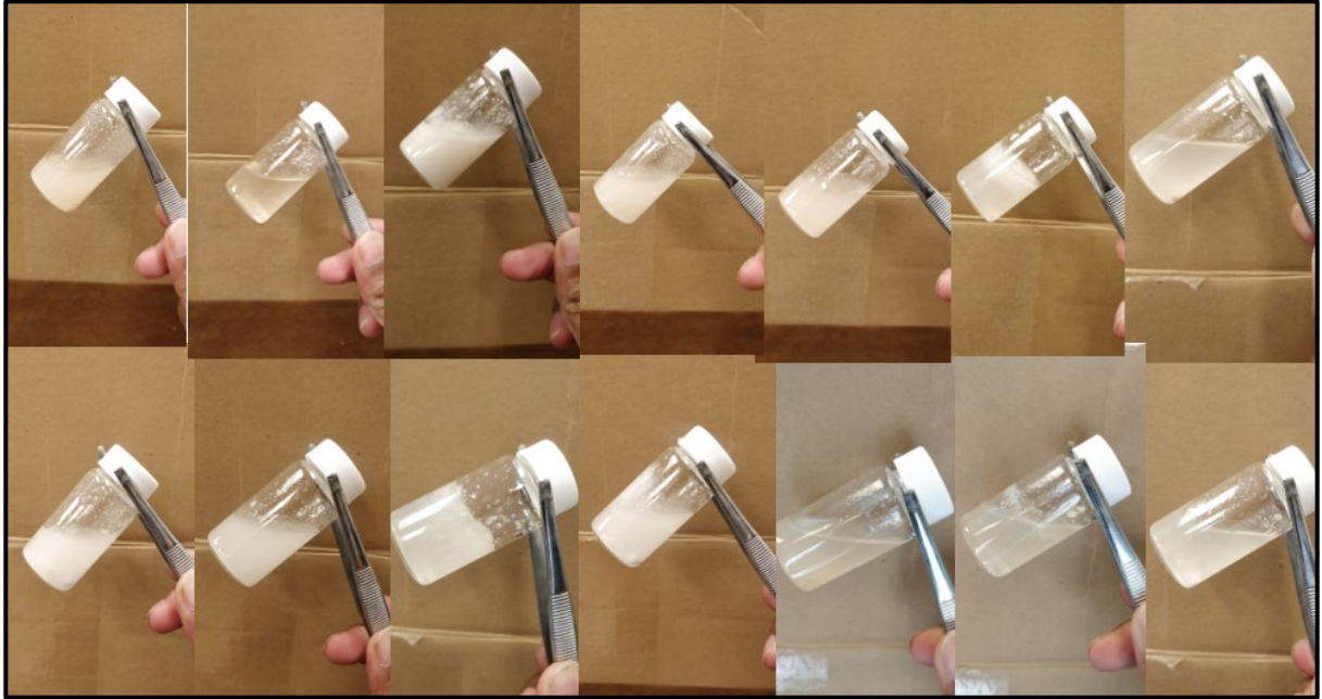
Figure 9. Manipulated formulations showing viscous gel which was not syringeable.
