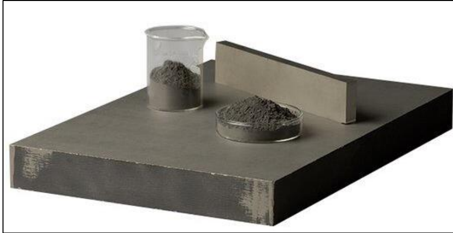
FIGURE 4: POWDER AND POLYCRYSTALLINE TiB2 [28]
