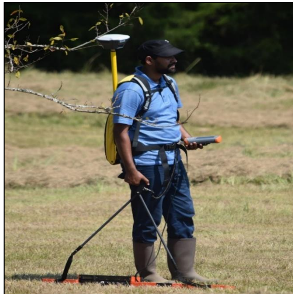
Figure 3.3: EM survey to detect soil collapse features.
