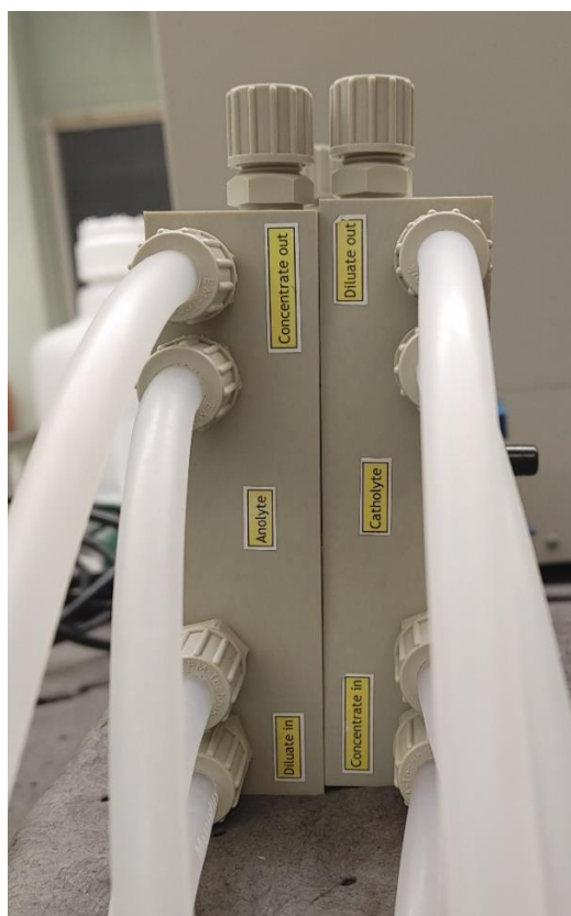
Figure 2-1. Photo of ED system used with concentrate and diluate streams labeled.
