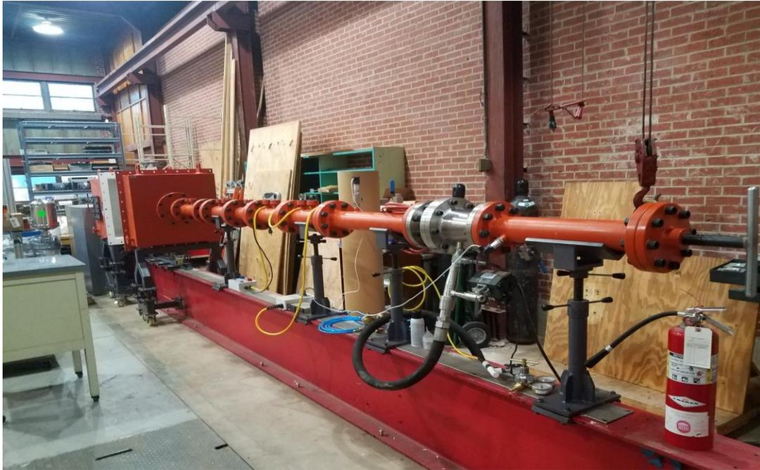
*Figure 31. Variable Pressure Shock Tube (Srushti Engineering Innovations PVT. LTD., 2020)*
