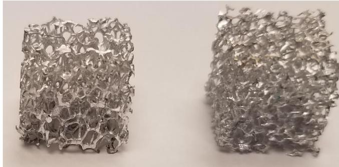
*Figure 23. Quasi-Static Compression and Split Hopkinson Pressure Bar Metallic Foam Samples*
