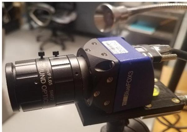
*Figure 24. mvBlueFox 3-2 2.4 Mpixel USB Camera*
