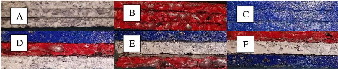
*Figure 67. Cymat Non-Functionally Graded (A-C), Functionally Graded (D-F) Low Velocity Impact Panels*
