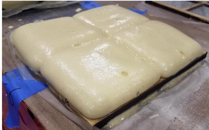
*Figure 19. Excess Polyurethane Foam on Composite Panels*
