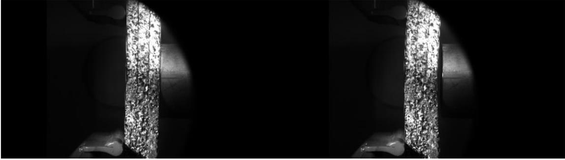
*Figure 131. Cymat Highest Density Configuration High Speed Images During Shock Loading*
