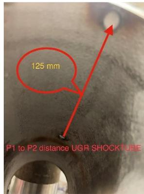
Figure 33. (A) Transducer Location Schematic, (B) Shock Tube Transducer Location
