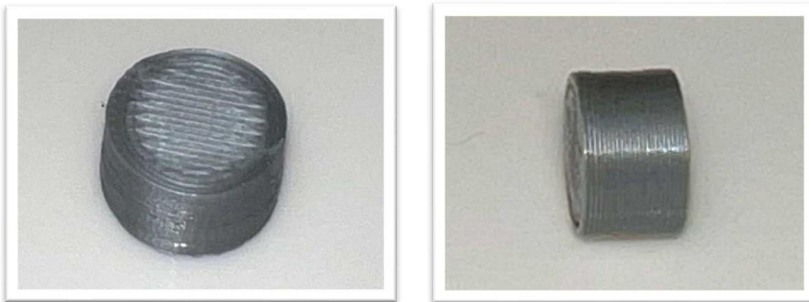
**Figure 6:** The Floating tablet design using PLA filaments through an FDM 3D printer.
