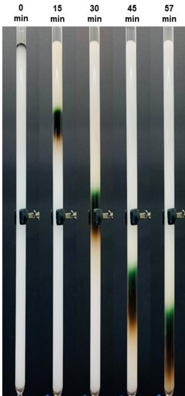
Figure S6.1. Time dependent photos of short SEC column during elution of etching product containing \text{Au}_{30}(\text{S-}t\text{Bu})_{18} at 7514 Da, \text{Au}_{46}(\text{S-}t\text{Bu})_{24} at 11200 Da and \text{Au}_{65}(\text{S-}t\text{Bu})_{29} at 15389 Da.
