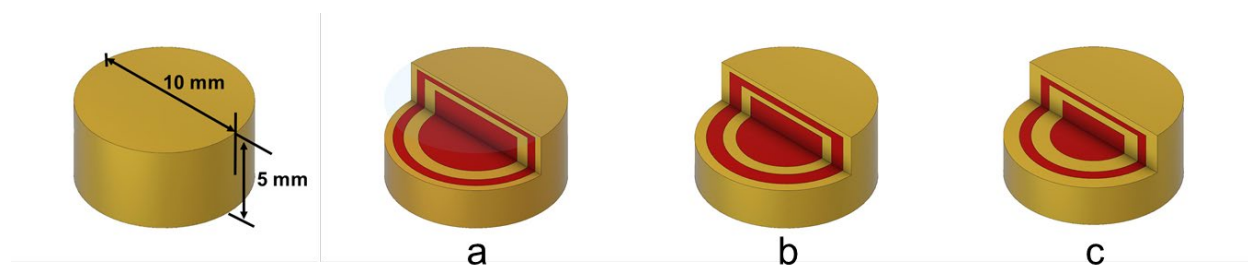
Figure 3.1. The 3D designed models of pulsatile-released tablets. a) 1:1:1:1 ratio of volume; b) 2:2:1:1 ratio of volume (outside in); c) 4:2:2:1 ratio of volume
