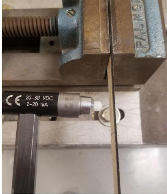
**Figure 9.** Tapping the specimen at the proper location in accordance with the desired FRF matrix element
