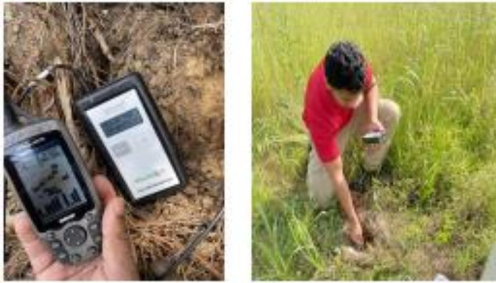
**Figure 6.** Soil moisture data collecting using the field soil moisture sensor. (LEFT) in closeup of the instrument interface along with a handheld GPS unit, and (RIGHT) showing position of probe in prepared test excavation.
