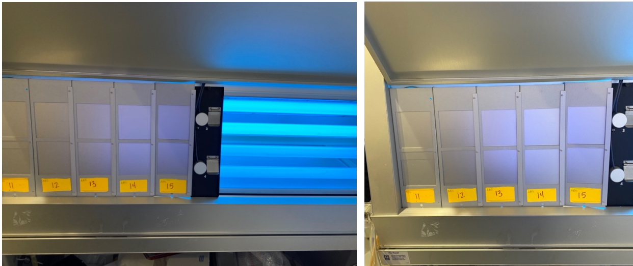
Figure 3. ABS Samples Loaded in QUV Accelerated Weathering Tester
