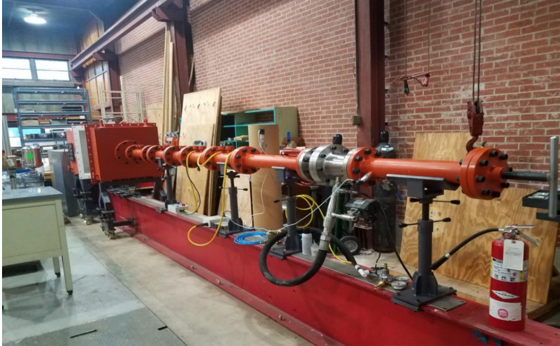
Figure 6. Variable Pressure Shock Tube
