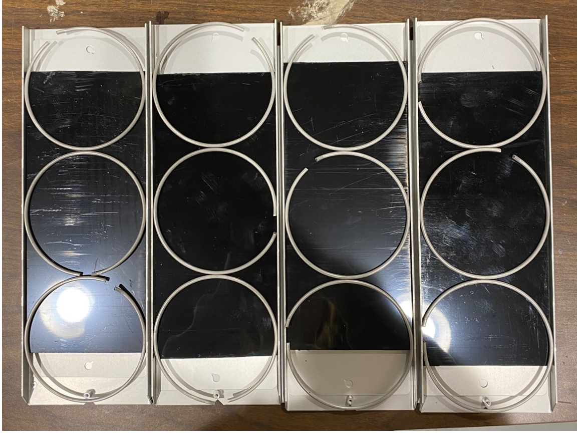
Figure 4. ABS Samples Loading Mechanism
