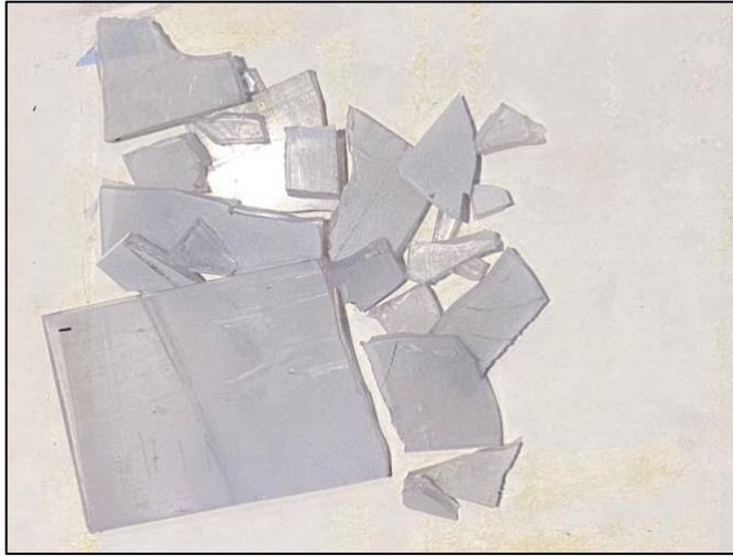
Figure 10. Unconditioned Polycarbonate Samples After Shock Tube Test
