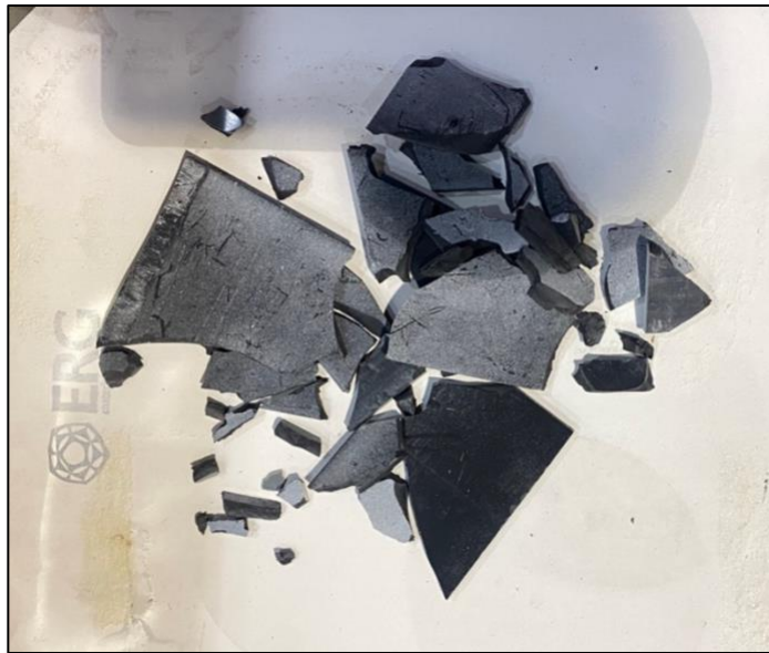
Figure 11. Unconditioned PVC Samples After Shock Tube Test
