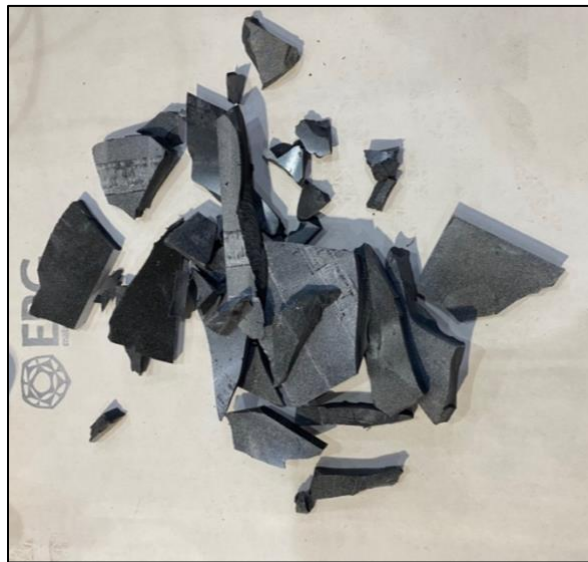
Figure 13. Conditioned PVC Samples After Shock Tube Test
