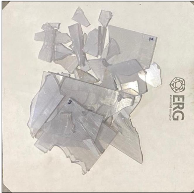
Figure 12. Conditioned Polycarbonate Samples After Shock Tube Test
