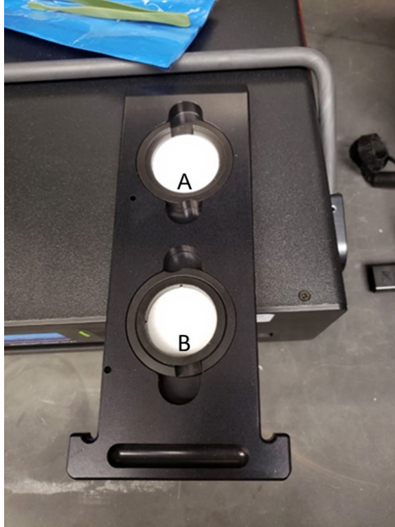
Figure 2: Sampling tray for the SootScan Transmissometer Blank filters (A) were compared to the sample filters (B) in this holding tray that was placed into the SootScan instrument for black carbon analysis at 880 nm.
