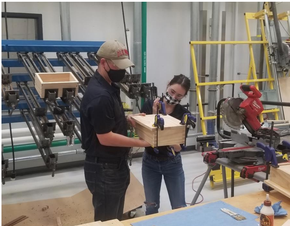
Figure 19: Team Demonstration on How the Lid is Glued and Clamped
