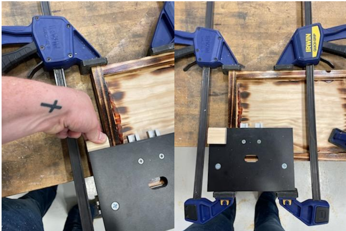
Figure 15A and 15B: 1.5" Hinge Slot Measuring Block
