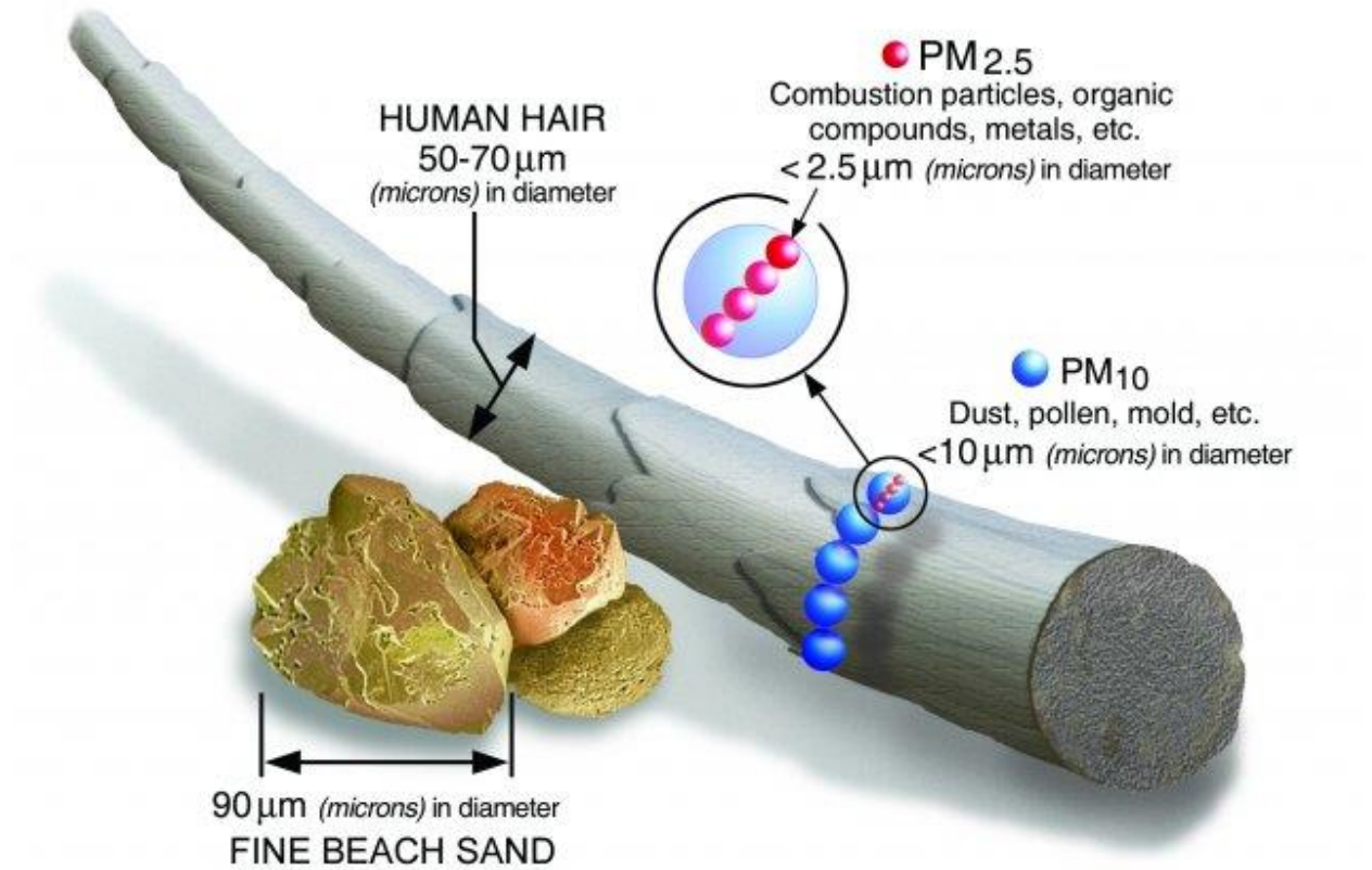
Figure 1: The size of PM 2.5 compared to a human hair US EPA, O. (2016b, April 19). Particulate Matter (PM) Basics [Overviews and Factsheets]. https://www.epa.gov/pm-pollution/particulate-matter-pm-basics
