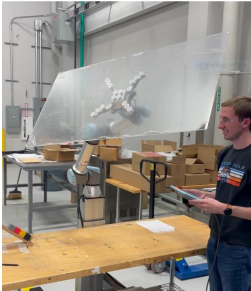
Figure 15: Collaborative Robot VG10 Gripper Setup
