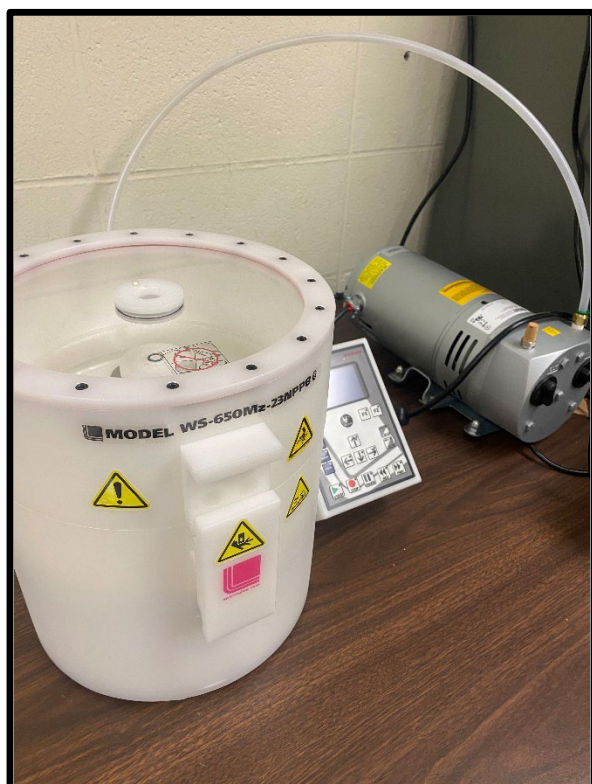
Figure 15: Spin-coater with QCM-D sensor attachment and vacuum pump experimental set up.
