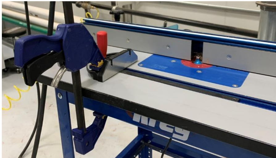
Figure 14: Router setup showing backstop and side stop for cord channel
