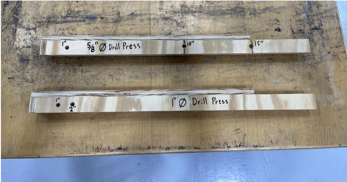
Figure 14: Drill Press Jigs
