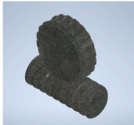
Figure 25: Worm and Worm Gear. Inventor Drawing by Lydia Miller and Jacob Schwartz. The worm to worm gear torsional ration is 1:20. The diameter of the worm gear is 1.8 inches and the height is 0.6 inches. The length of the worm is 2.36 inches.
