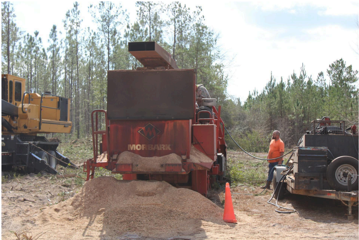
Pictured is a $700,000+ wood chipper, belonging to the Timberline Forestry, LLC, which helps turn cut pine trees into wood chips. These wood chips are sold to various companies, who in turn produce lumber-based products. Photo by Kala Nance.
