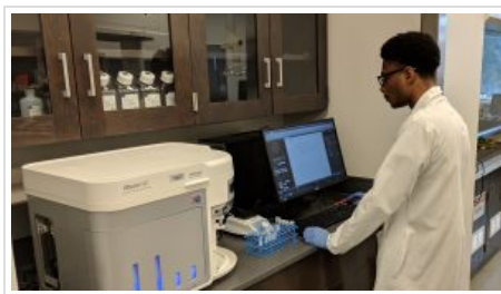
Larry Stokes, a former undergraduate member of the Interdisciplinary NanoBioSciences Lab at the University of Mississippi, runs a flow cytometry analysis on cells being used in the lab. Submitted photo
