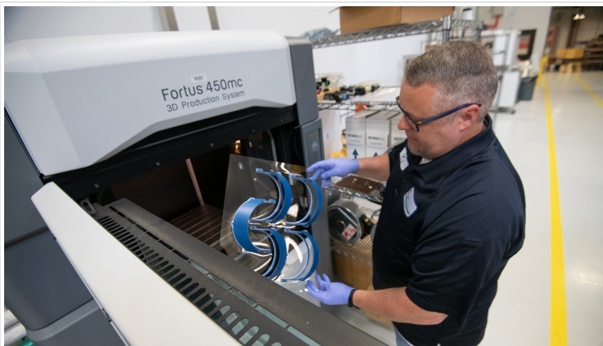
Andy Gossett, a technical support staff member at the UM Haley Barbour Center for Manufacturing Excellence, removes a batch of 3D-printed headbands from one of the facility's printers. The headbands will be used for face shields by health care workers at Baptist Memorial Hospital-North Mississippi in Oxford during the COVID-19 pandemic. Photo by Kevin Bain/Ole Miss Digital Imaging Services
